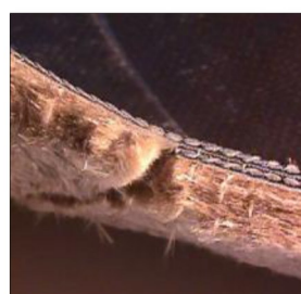
Photographs showing Discontinuous Barriers (fluid and thermal) in the THERMALAM ™ Expansion Joint Product Using Conventional Bias Construction Technology.
